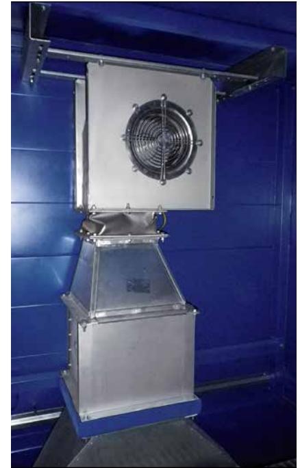
Electric air recirculation heating with digital temperature regulation
