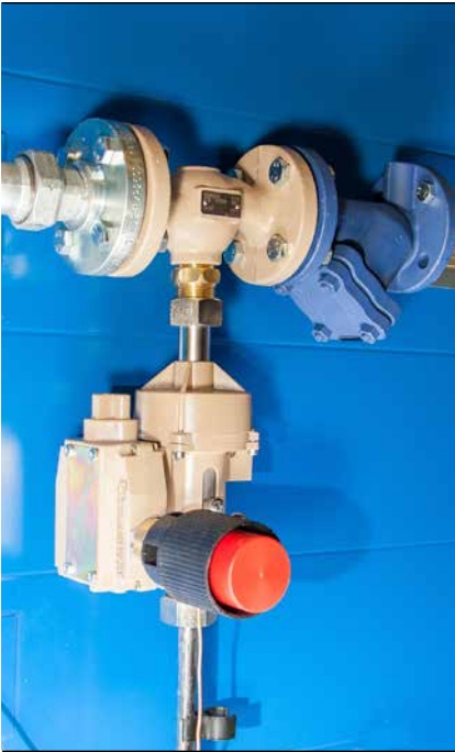
Steam heating with temperature regulation, mechanical, without auxiliary power
