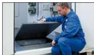
Double floor with inspection flap for technical equipment
