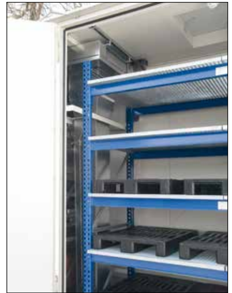
Racking system for optimised storage of batteries on carriers
