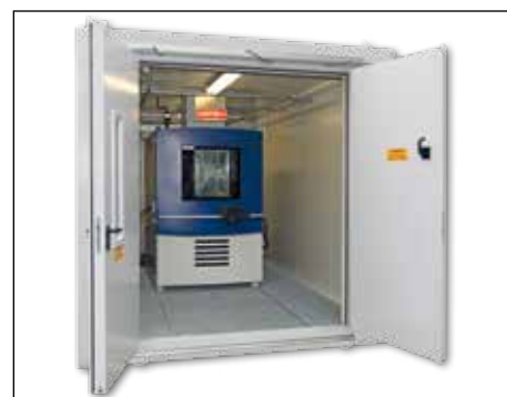
Walk-in F90 fire-rated container with integral climate chamber
