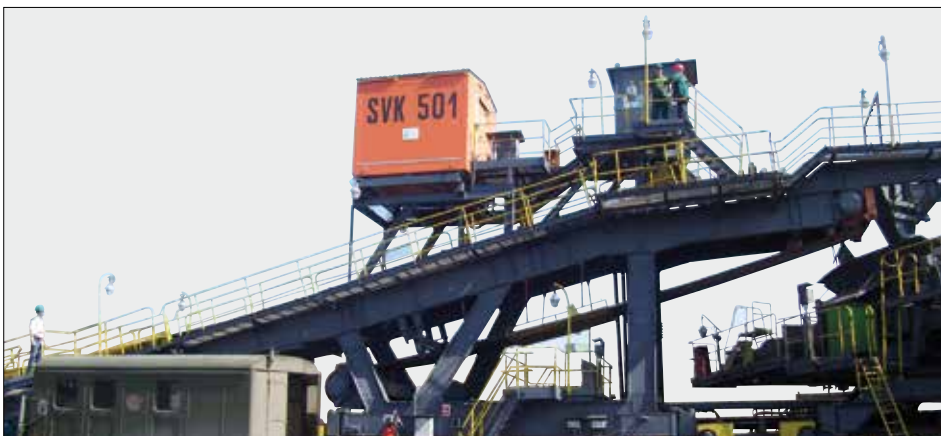
Technical / safety room with transformer in brown coal surface mine
