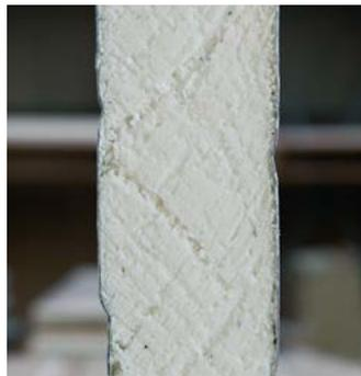
Section through flame-retardant PUR panels (building material class B)
