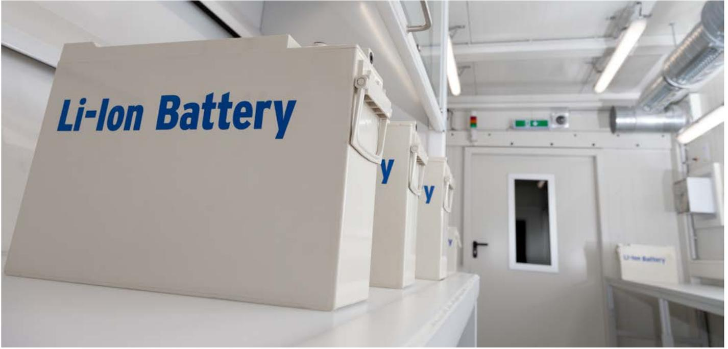
The AT Li-Ion worktable offers the highest level of personal safety during testing procedures on lithium-ion batteries. A water basin integrated into the table and a smoke extraction system provide immediate evacuation of the working area in case of battery failure. Due to its sturdy construction, the worktable is optimally designed for use in a tough industrial environment and is also ideal for use in a laboratory.
