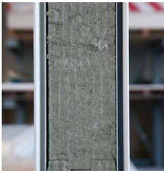
Section through non-combustible mineral wool panels (building material class A)
