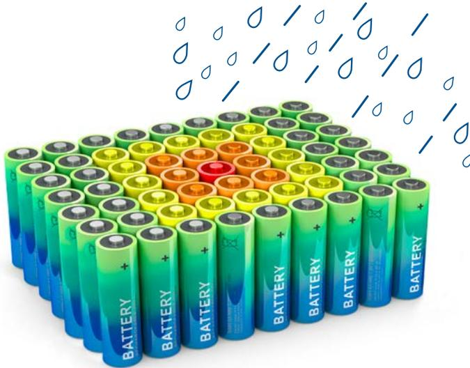
Schematic structure of a **larger**, failing battery module and water cooling
